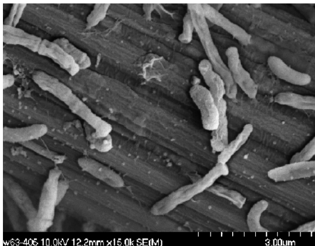
Fig. 3. SEM image of electron-transfer bacteria attached to the surface of the anode.
